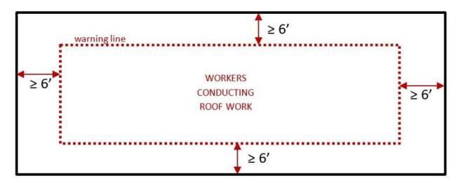
Warning lines can only be used on low-sloped roofs. A low-sloped roof is one that has a slope no greater than 4:12 (vertical:horizontal). Additionally, there are specific requirements based on the type of work being performed on the roof.
